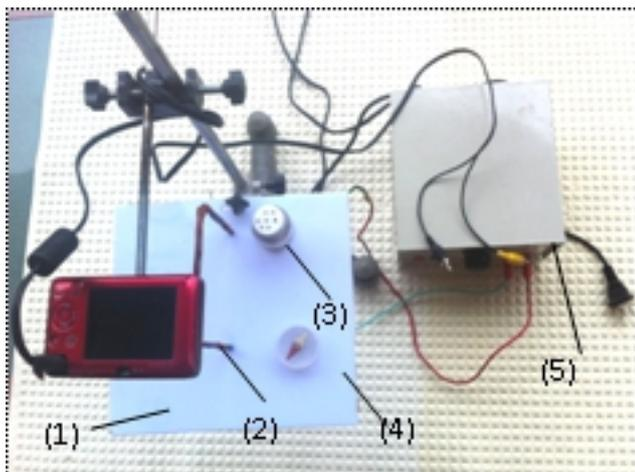
Figure2: Surveying the magnetic fields of a cussent in a long straight
